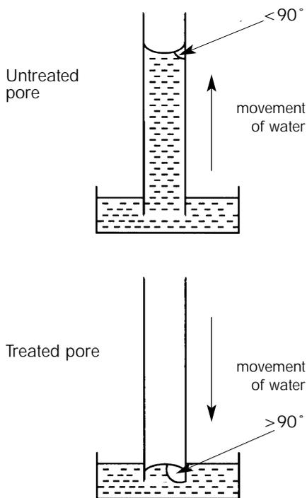
**Figure 7:** Fingering effect of pressure injected DPC fluid
