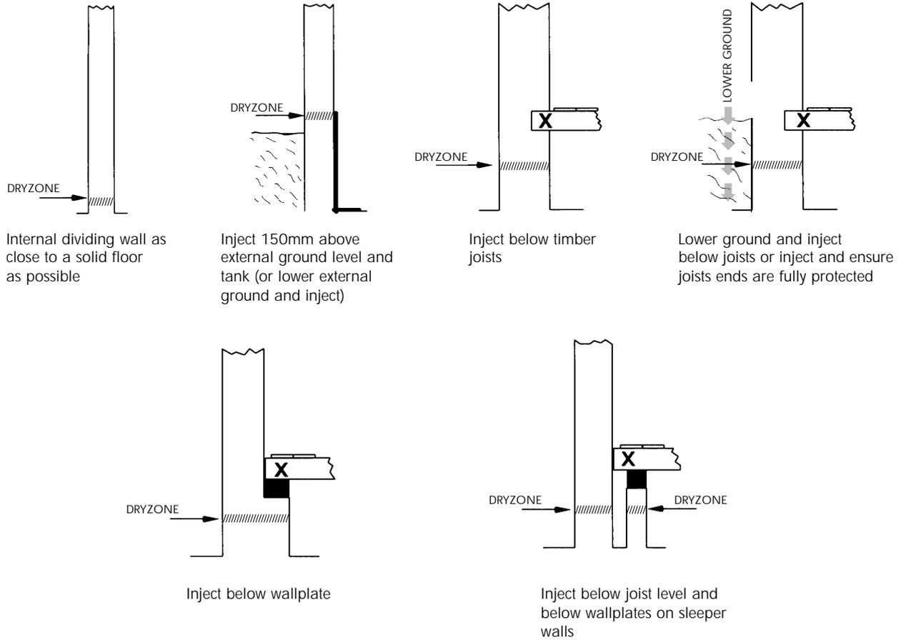
'X' = all timber should be preferably physically isolated from any damp masonry in the vicinity of the DPC. Where this is not possible fully treat timbers with Safeguard ProBor 50 in accordance with the directions given in the Safeguard 'Dry rot and its Control' publication, available free from [www.safeguardchem.com](http://www.safeguardchem.com)
